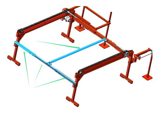
Install the middle reinforcement connecting pipes.
