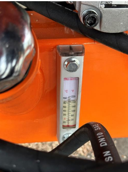
FIG 18: the Hydraulic oil should be always full. This is the minimum oil requirement on this picture.
